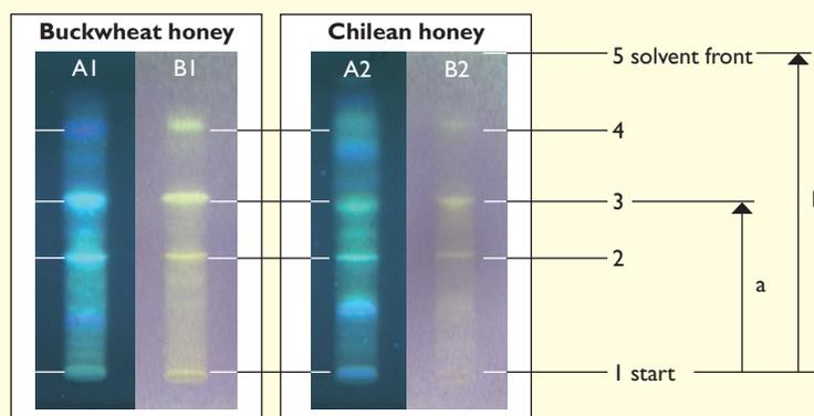
A = Detection with natural product reagent, showing flavonoids and other phenolic components as green and blue fluorescent spots under ultraviolet light of 366nm
